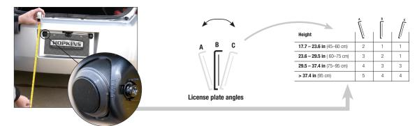
**4)** For camera (B), adjust the angle up/down to create maximum visibility behind your vehicle.
