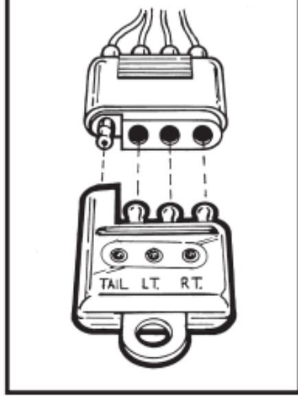
Plug into tow vehicle side to check all connections. LED lights will confirm that each connection is operating.
