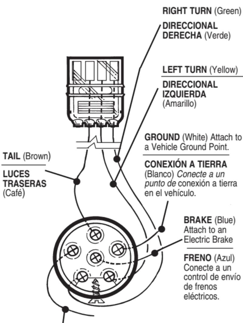
**BATTERY (Red)** Auxiliary Power Lead. Connect to **Fuse Block** or **Fused Battery Lead**.
